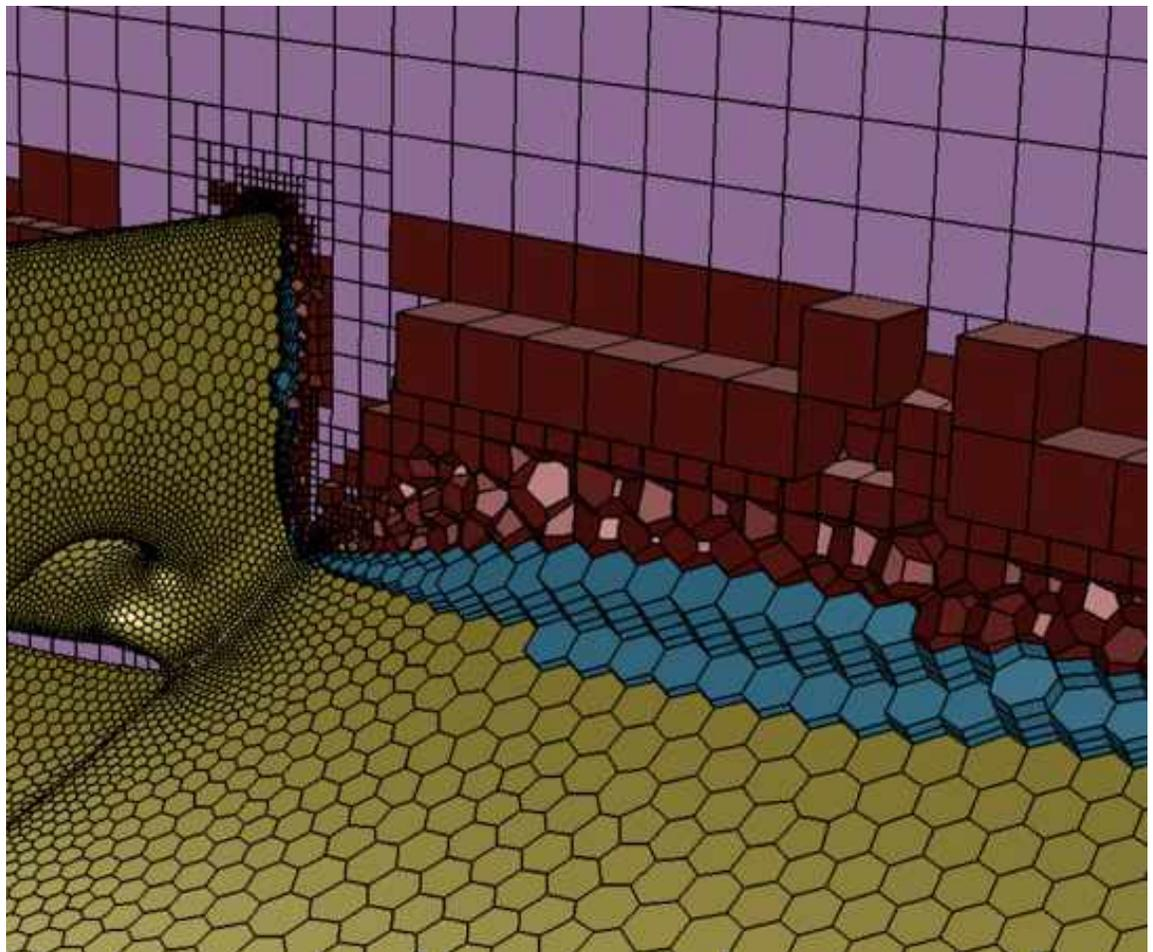
Mosaic meshing technology conformally connects hexahedral elements in the bulk region and isotropic elements in the boundary layer with polyhedral elements.
